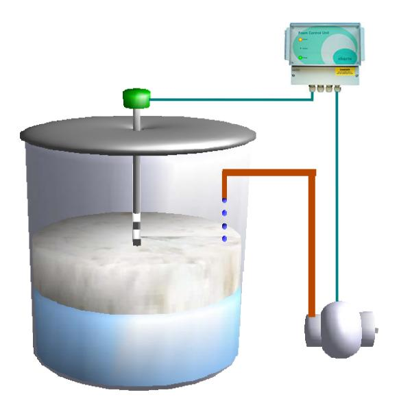
Because the Sensor and Controller are very sensitive to levels the antifoam is added on an 'as required' basis, thus regulating the amount of antifoam used and giving a significant cost saving.
