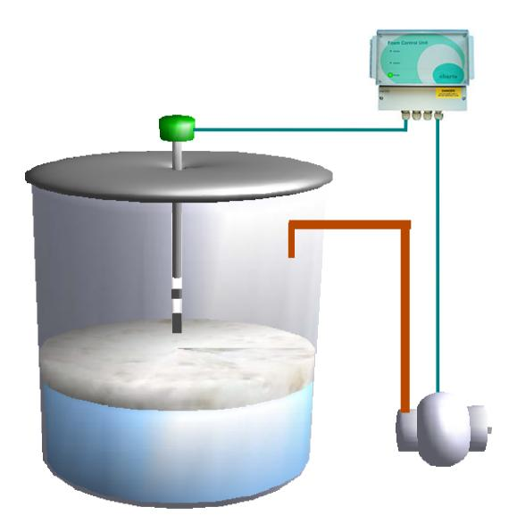
As the process begins foam starts to be generated on top of the liquid.
