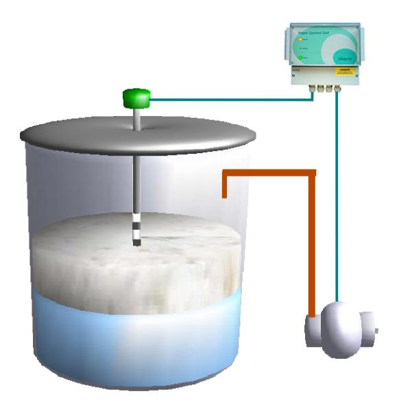
As the foam level increases the Sensor signals back to the Controller that foam has been detected. The Sense light illuminates on the Controller to indicate the increasing level of the foam.
