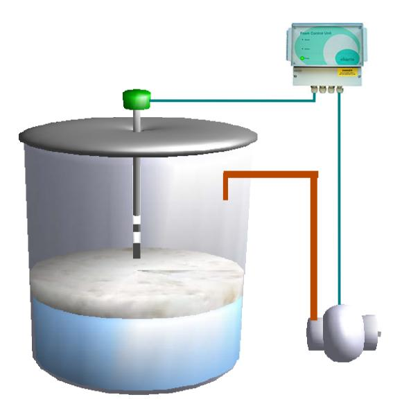
With the level of foam now returned to normal the antifoam pump has stopped, leaving the Charis Sensor and Controller on standby until the cycle starts again.
