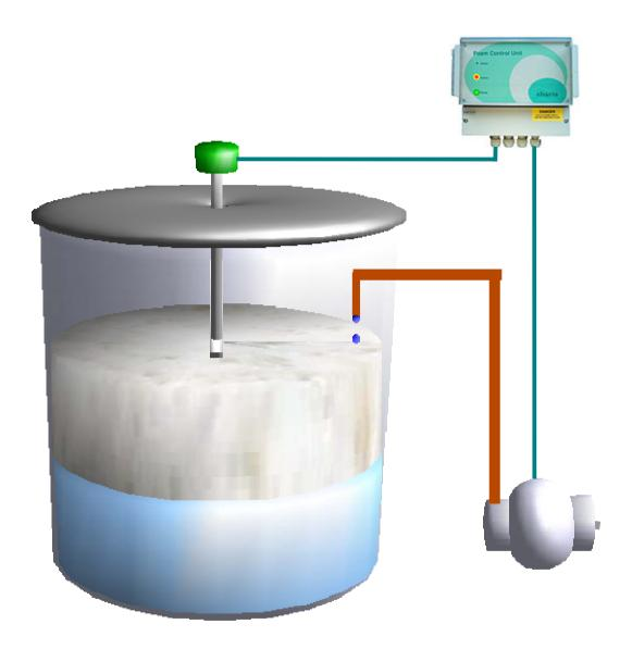
When the foam reaches a pre-set level the Sensor signals the Controller to start adding anti-foam. The Activate light on the Controller illuminates to indicate that action is being taken to reduce the foam.
