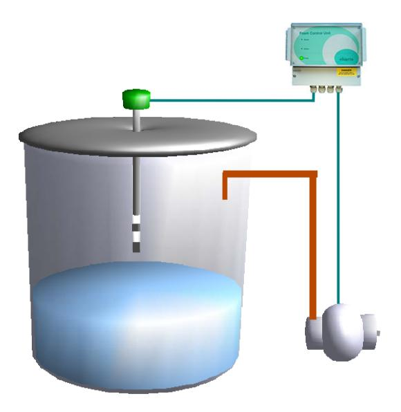
A Charis Foam Sensor is fitted through the top of a fermenter vessel. The sensor is connected to a Charis Foam Controller, which in turn is connected to a pump controlling the flow of antifoam into the vessel.
