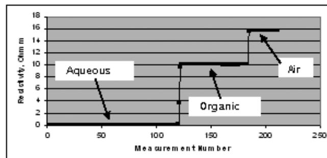
Figure 6: Interfaces between different materials flowing through sensor
