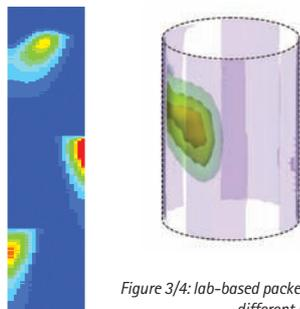
Figure 3/4: lab-based packed bed and spreading of brine pulses at different positions in packing.
