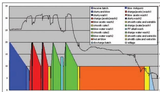
Figure 1: Process cycle vs tomography signal
