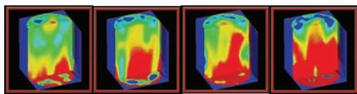
Figure 3: Effect of sparging rate on gas distribution. Red regions indicate gas concentrations greater than 15% v/v
