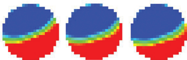
Figure 2: Cross-sectional conductivity tomographic images for 40, 50 and 60% oil.
